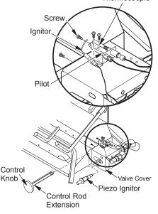
Figure 13 - Installing Cover, Control Knob and Piezo Ignitor
